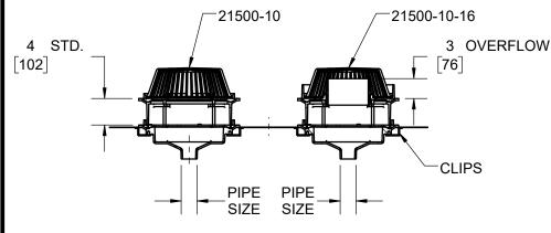
PRIMARY DRAIN OVERFLOW DRAIN
